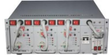
**MODEL DY 3700DRC is a Modular Power System, which uses 3 nos. Hot-Pluggable DY 700D Rectifier Modules of 700Watts and a detachable additional Controller to ensure break-free System operation.**
