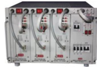
**MODEL DY 31400ERC is a Modular Power System, which uses 3 nos. Hot-Pluggable DY 1400E Rectifier Modules of 1400Watts and a detachable additional Controller to ensure break-free System operation.**
